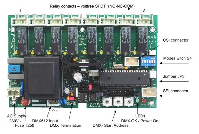
The DSP8 is a DMX512 controlled 8 channel Relay switchboard. Each relay contact is able to switch 230V~/ 8A continues- and 30A inrush current. ( At resistive load, AC1, only)
