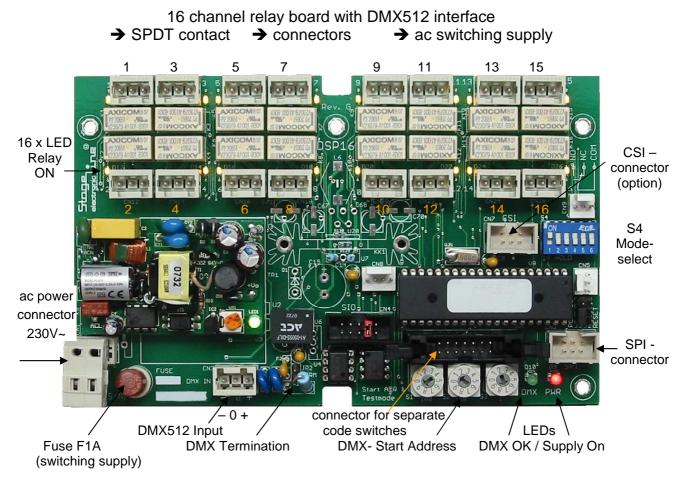
The DSP16 is a DMX512 controlled 16 channel relay switchboard. Each relay contact is able to switch 42V=/~, 2A continues- or inrush current.
